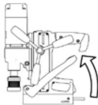
When drilling is complete, simply release the lock & remove the MAGRIG
