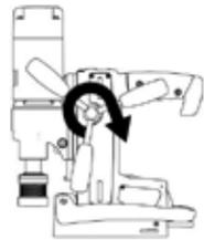
Turn on the drill & slowly rotate the handles to drill into the safe.
